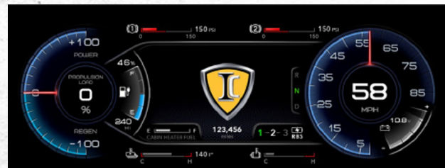
The Electric CE Series features a state-of-the-art digital gauge cluster for easy readability, and coaching for efficient driving.
